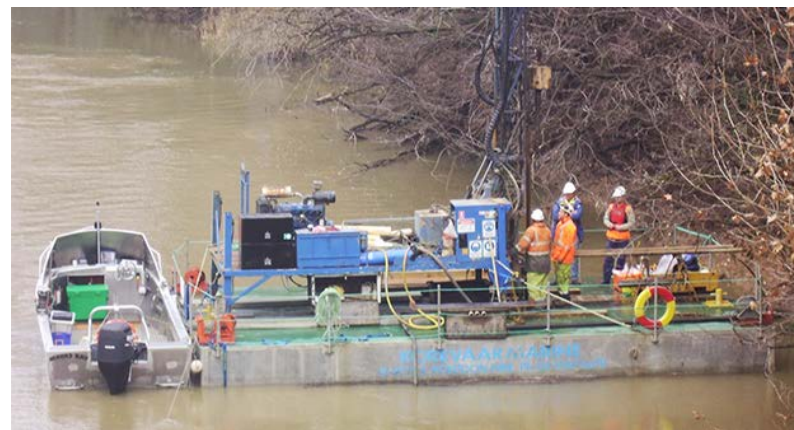
10m Aluminium pontoons carrying out geophysical testing on the Ovens River, Wangaratta, Victoria
