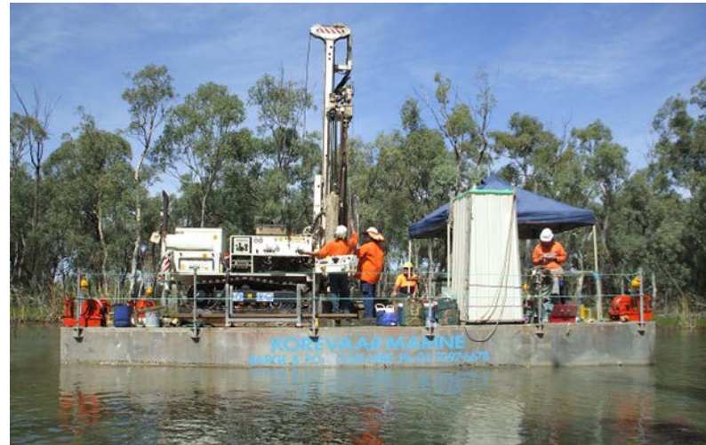
10m Aluminium pontoons carrying out Geophysical testing on the Gunbower Creek, near Cohuna, Victoria
