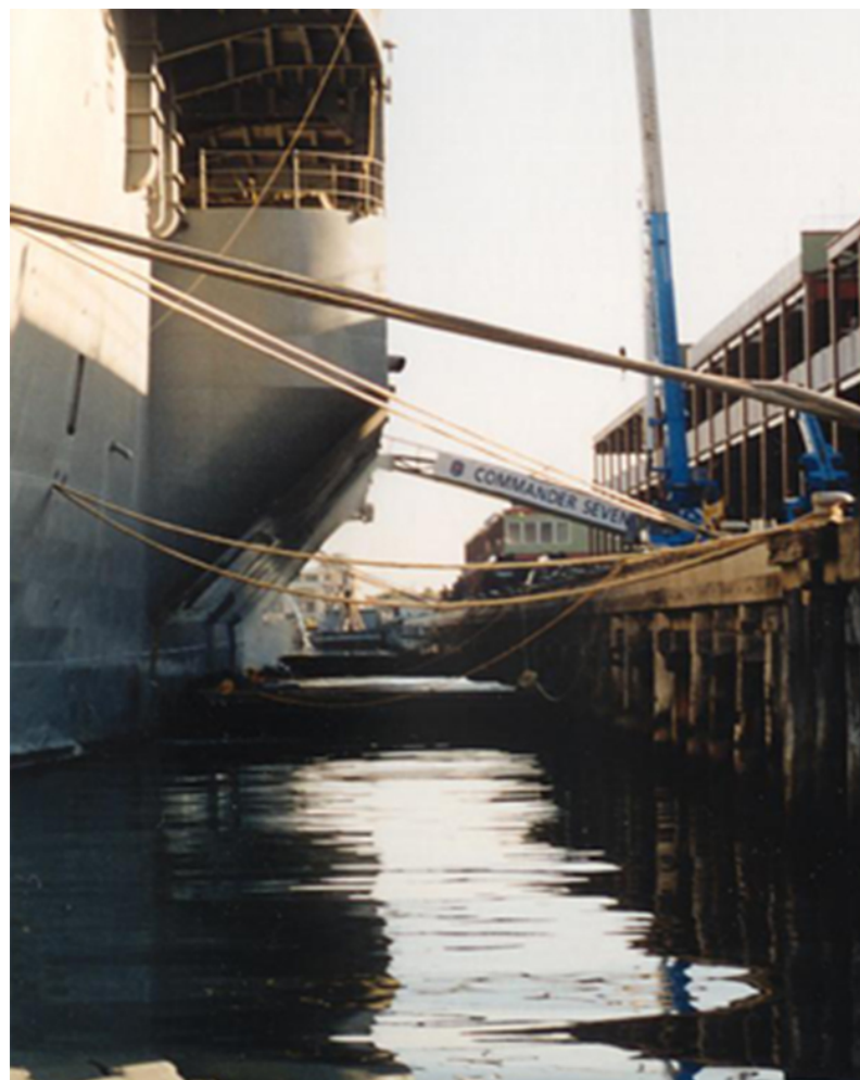
6m Steel Pontoons in use as breasting barges for navy ship at Station Pier, Melbourne
